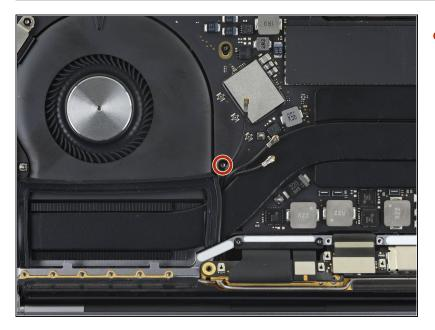
• Remove the 2.8 mm T5 Torx screw securing the three antenna coax cables to the main board.
