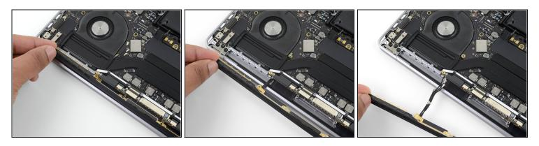
• Carefully remove the antenna assembly, while simultaneously feeding the antenna cable bundle out from underneath the heat pipe.
