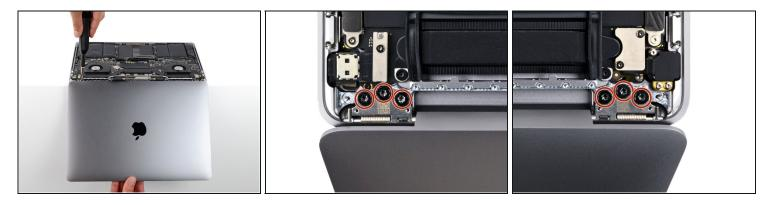
• Support the screen with one hand and use your free hand to remove the six T8 Torx screws securing the hinges.
