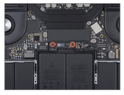
Use a T5 Torx driver to remove the two 3.2 mm screws from the battery board.
