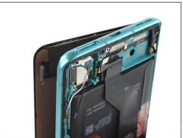
Thread the display flex cable through the gap in the frame.
