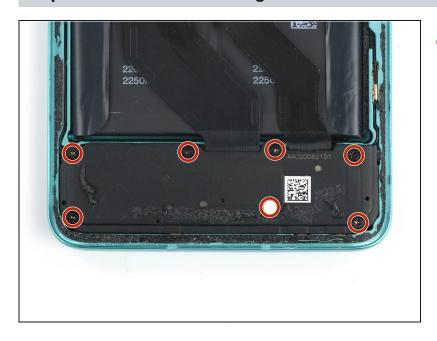
Use a Phillips screwdriver to remove the seven 3.8 mm-long screws securing the daughterboard cover.
