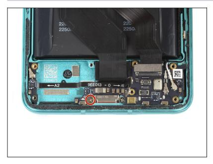
Use a Phillips screwdriver to remove the 3.1 mm-long screw securing the daughterboard.
