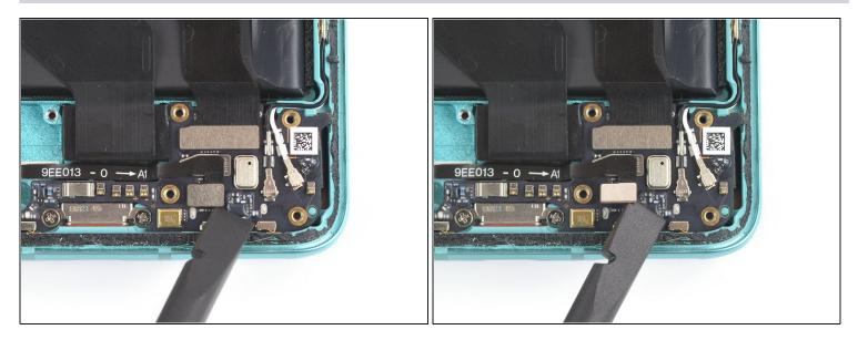
Use a spudger to disconnect the first fingerprint sensor connector by prying it straight up from its socket.
