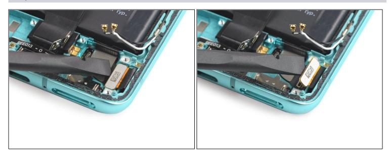
• Use the flat edge of a spudger to pry up and disconnect the screen connector from its socket at the frame.
