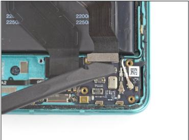
Use a spudger to disconnect the interconnect cable by prying the connector straight up from its socket.
