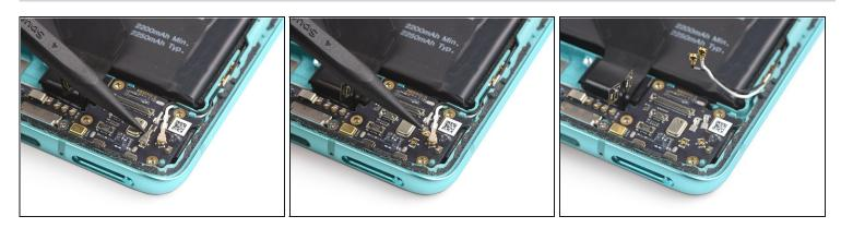
Carefully disconnect the two antenna cables by prying them straight up from the daughterboard.
