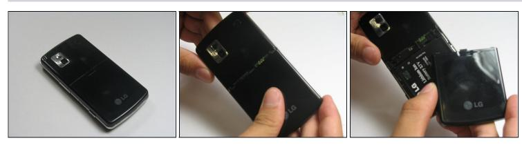
• Remove the back cover by firmly pressing against the indent on the back panel. Slide the cover downward and off the phone.
