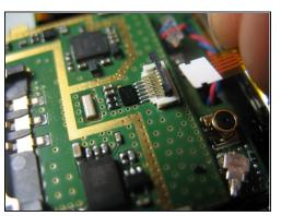
• Gently lift the ZIF connector (black tab) holding the ribbon cable in place. When it is in the upright position, remove the cable from the back side.
