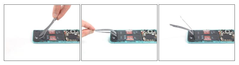
• Bend the two flex cables toward the bottom of the phone and out of the way of the battery.
