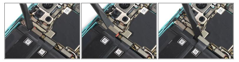
• Use the flat end of a spudger to disconnect the two flex cables which are covering the battery.
