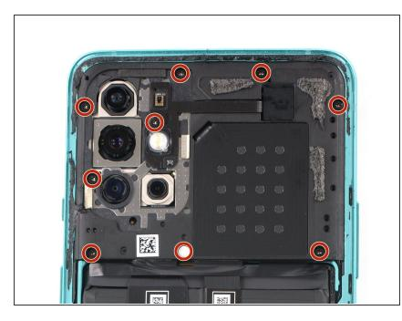
Use a Phillips screwdriver to remove the nine 3.8 mm-long screws securing the motherboard cover.
