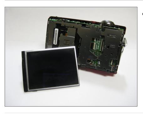
Disconnect the LCD screen from the logic board!
