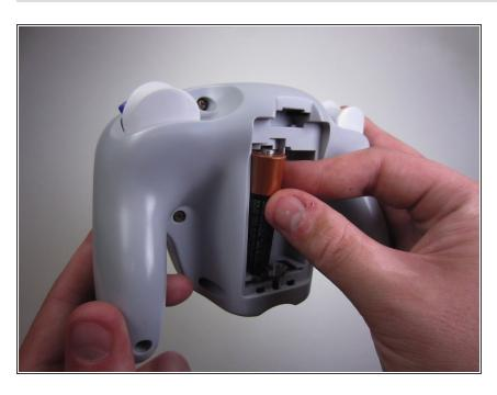
Remove both batteries from the device.
