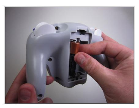
• Remove both batteries from the device.
