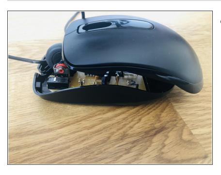
Applying some force lift the mouse top up and backward at the same time to disconnect it
