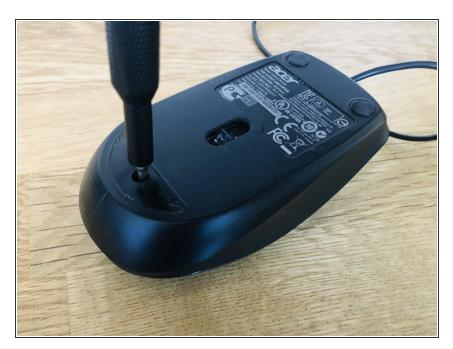
Using a phillips #0, unscrew the screws
