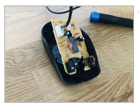
Pull on the cable and the board should come out
