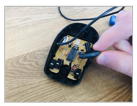
Once inside pull on the scroll wheel to remove it from the board
