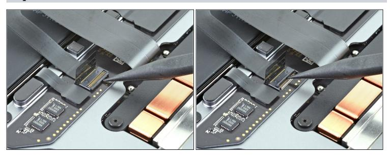
• Use the pointed end of a spudger to lift up the small locking flap on the trackpad cable's <u>ZIF connector</u>.
