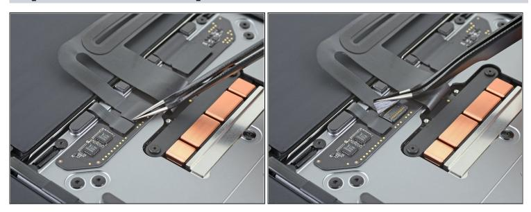
• Use a pair of <u>tweezers</u> to peel back the tape covering the trackpad cable connector.
