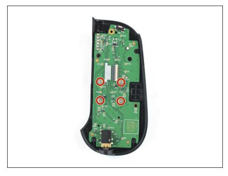
Use a Phillips screwdriver to remove the four 3.9 mm-long screws.
