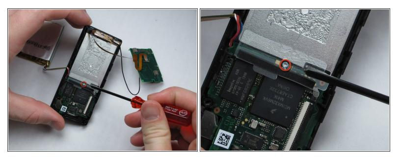
• Remove the single screw under the battery using a small Tri-Wing screwdriver.
