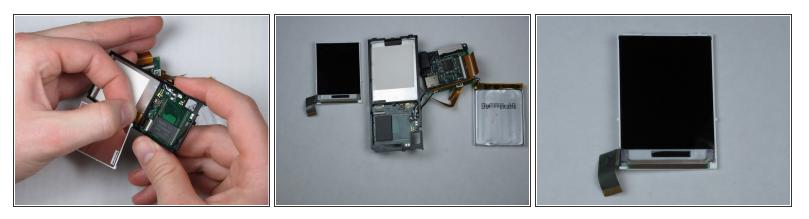
∧ The LCD ribbon is adhered to the memory board with a strip of glue.
