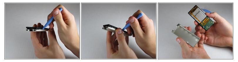
Work your way around the Zune until the back cover comes free. Remove the back plate and set it aside.
