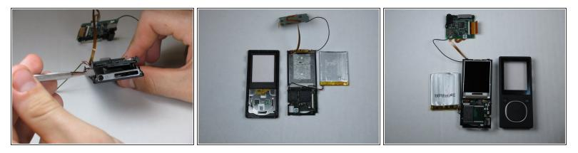
• Remove the faceplate by using a metal spudger to separate it from the remaining components.
