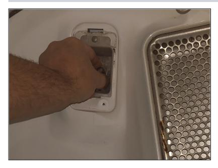
Unscrew the light from its base in the enclosure.
