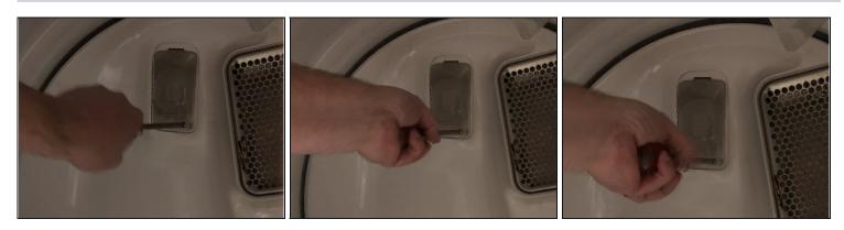
Remove the 14 mm long Phillips screw in the lower right of the light cover.
