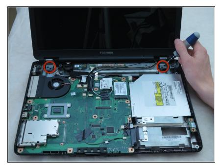
Using a Philips #1 screwdriver, remove the four 6-mm screws from the two metal tabs that connect the screen to the body.
