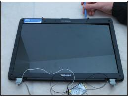
Using a plastic opening tool, pry off the top of the screen casing.
