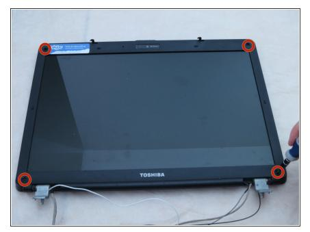
Using a Phillips #1 screwdriver, remove the four 4-mm screws at the corners of the screen.
