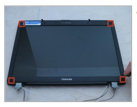
Using tweezers, pry the rubber feet out of the corners of the laptop.
