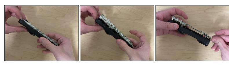
To remove the motherboard, press up on the "B" button, and then the connector at the bottom.
