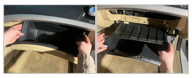
Push in on both sides of the glove box to locate the housing cover.
