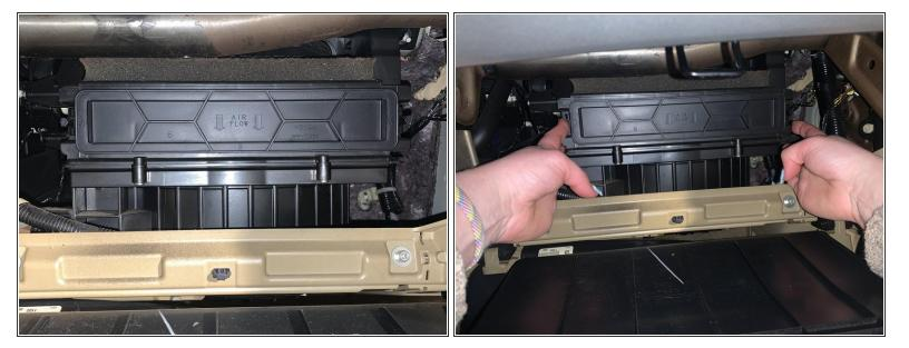
Unclip both sides of the housing cover to remove it.
