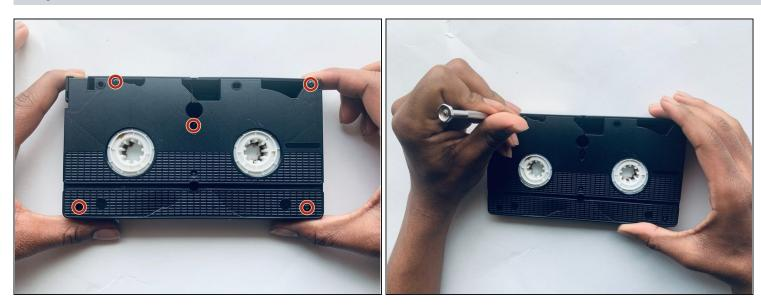
Unscrew the five 3mm screws with the Phillips #1 screwdriver.
