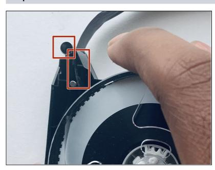
Place the left reel into the replacement shell, making sure the tape goes in-between metal circular piece and the plastic triangular piece pictured.
