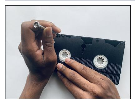
Screw the screws back in with a screwdriver.
