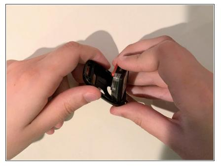
• Remove the inner shell from the outer shell by pushing the buttons to loosen the inner shell.
