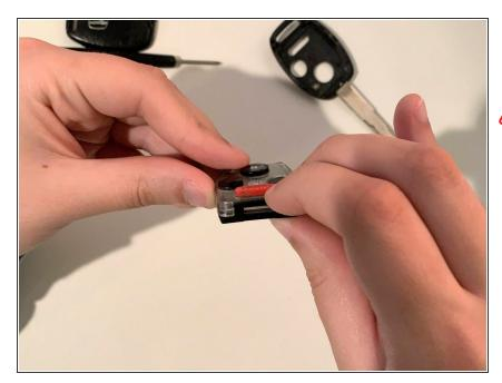
• Unclasp the inner shell using the clips on the top and bottom.
