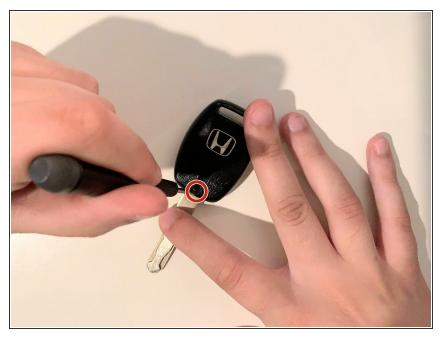
Using the Phillips #0 screwdriver, remove the single screw from the bottom of the key FOB.
