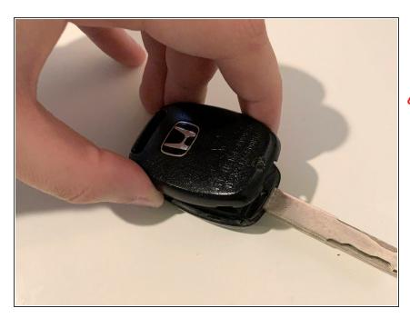
• Gently lift the outer shell and remove it from the rest of the device.
