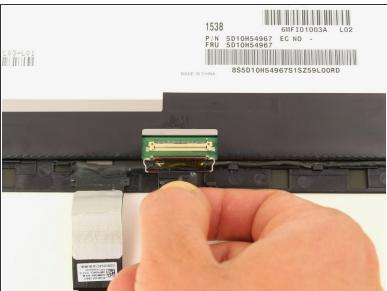
Pull the tape downward to unplug the display cable.
