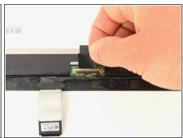
Peel up the small strip of tape wrapped around the locking bar of the display cable connector.
