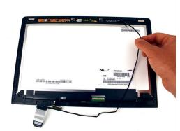
Gently pull the cable out from the routing to free it from the hooks along the edge of the screen.
