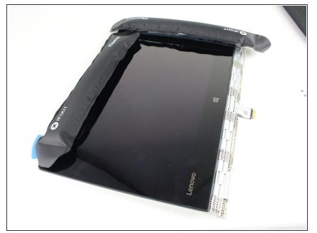
• Use a heat gun or iOpener to apply heat to the top and side edge that have not yet been opened.
