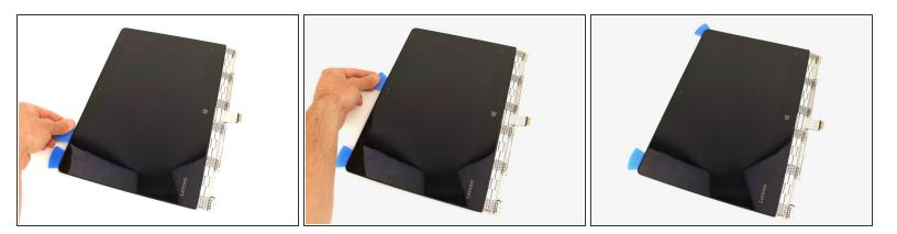
• Continue cutting away the adhesive on the top and side edges of the display.
