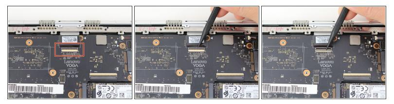
Use the pointed end of a spudger to lift the hinged locking flap of the display <u>ZIF connector</u>.
