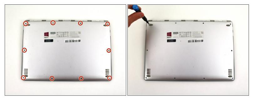
• Using a T5 Torx screwdriver, remove the ten 5.5 mm screws from the back case of the laptop.
