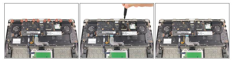
Remove the ten 3.6 mm screws from the hinge bracket with a Phillips #00 screwdriver.
