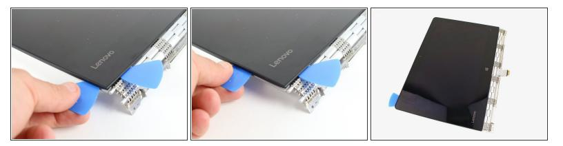
• Insert a second opening pick and slide it along the side of the display, cutting away the adhesive.
