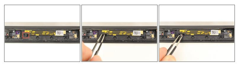
Gently remove the cable from the yellow-accented webcam board on the top of the display panel with a pair of blunt nose tweezers.
