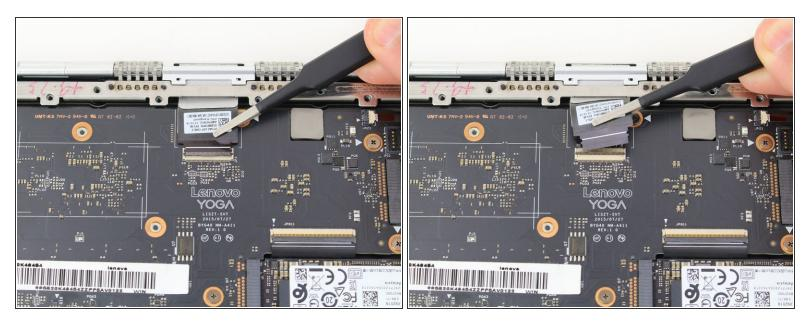
• Pull out the display cable with a pair of blunt nose tweezers.
