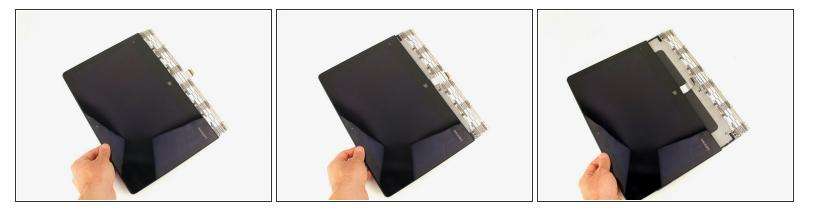
• Pull the display cable out from the hinge mechanism.
