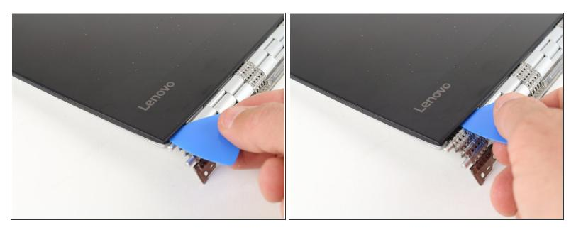
Insert an opening pick into the corner of the screen and slide it around slightly to create an opening.
