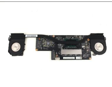
Flip the motherboard over to access the heatsink.
