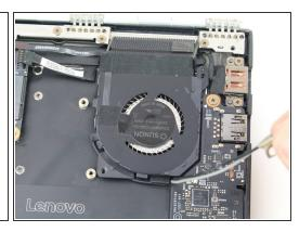
Unwind the black and white coaxial cables from the hooks on the right fan casing.
