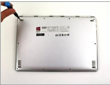
Using a T5 Torx screwdriver, remove the ten 5.5 mm screws from the back case of the laptop.
