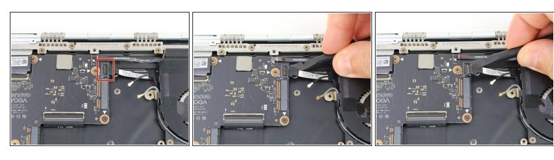
• Use a spudger to pry up the press fit connector on the right side of the motherboard.
