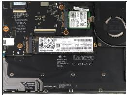
Use a Phillips #00 screwdriver to remove the 2.7 mm screw that is holding down the SSD card.
