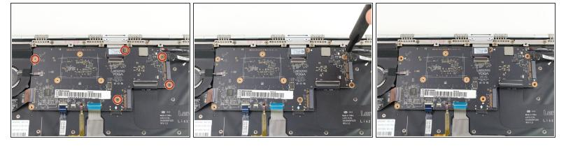
Remove the five 3.6 mm screws from the motherboard using a Phillips #00 screwdriver.
