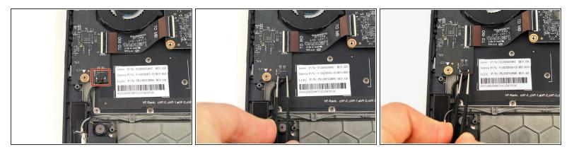
Use a pair of blunt nose tweezers or your fingers to pull out the speaker cable from the connector on the lower portion of the daughterboard on the left.
