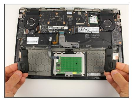
Continue unwinding the speaker cables from the hooks until the entire assembly is free from the case.
