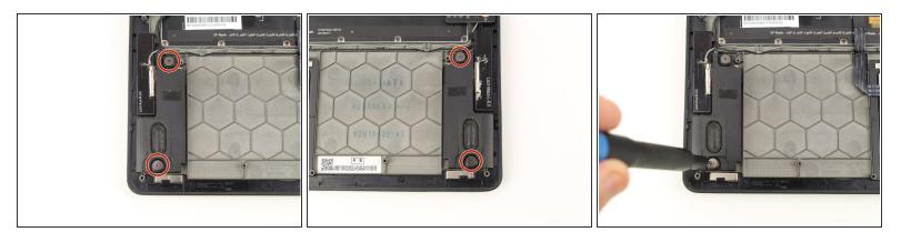
Remove the four 2.4 mm Phillips #00 screws from the speakers on either side of the case. (two screws per speaker)
