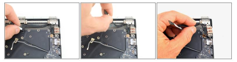
• Peel up the charging port cable and remove the charging port.
