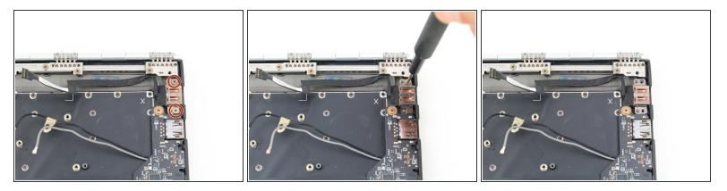
Remove the two 3.5 mm screws from the charging port with a Phillips #00 screwdriver.
