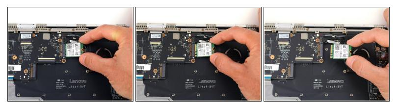
• Pull the WiFi card out from the connector on the motherboard.
