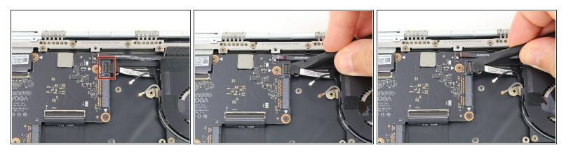
• Use a spudger to pry up the press fit connector on the right side of the motherboard.
