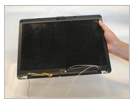
Once all the wires are detached and screws are removed, pull up on the monitor to remove it.
