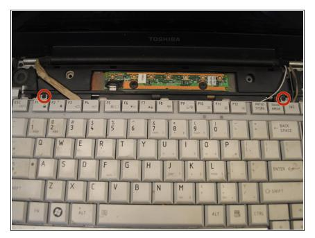
• Remove the two 4mm flat-head screws indicated in the photo.
