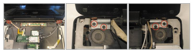
Remove the four 8mm button-head screws that are located in the top right (2) and top left corners
