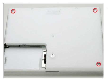
Remove the three newly-revealed Phillips screws.
