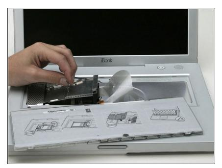
Grasp the metal bracket on top of the RAM shield and pull upward to remove the shield.
