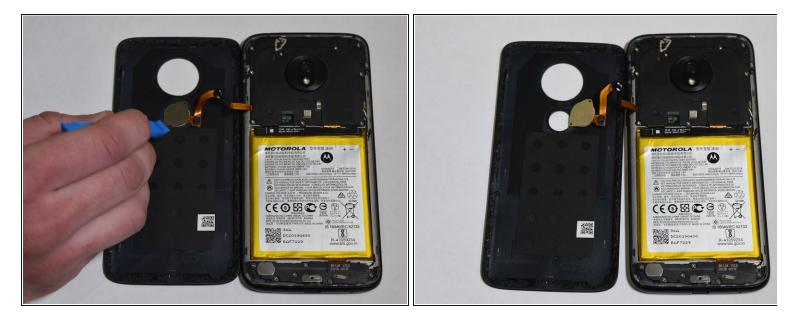
• Use the iFixit pick and the iFixit opening tool to pull the fingerprint scanner off of the back case.
