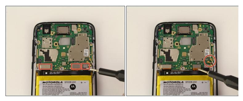
Once the motherboard cover is removed, disconnect the four ribbon cables and the two wires attached to the motherboard.
