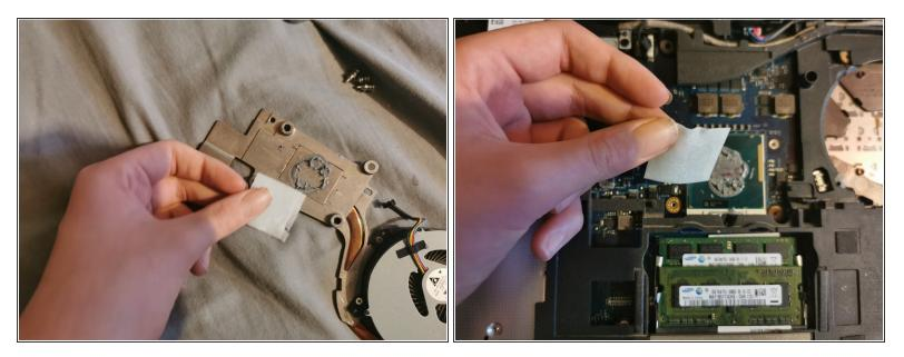
• Use a paper towel or alcohol swab to clean the thermal paste from the heatsink & CPU.
