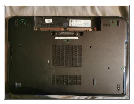
• Remove the 4 Philips #0 screws from the laptop.
