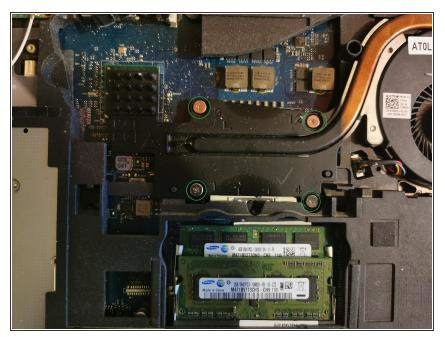
• Remove the 4 Philips #1 screws on the heatsink.
