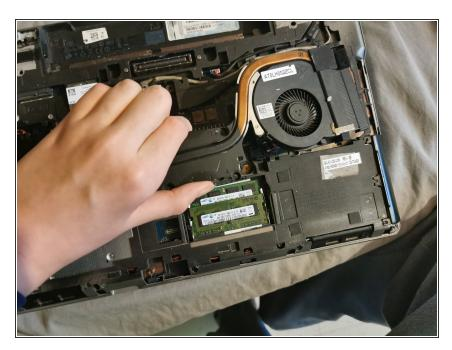
• Remove the Fan+Heatsink assembly.
