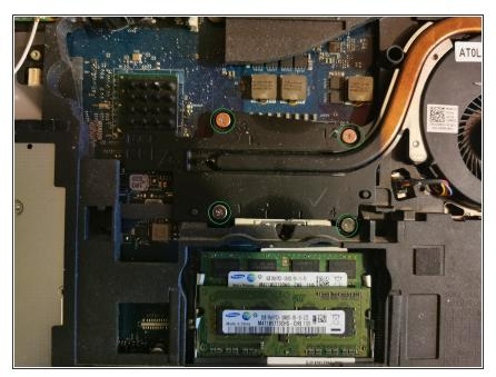
• Remove the 4 Philips #1 screws on the heatsink.
