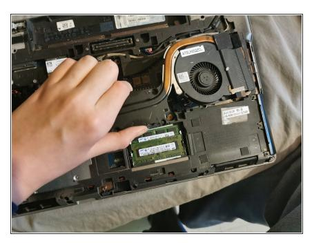
• Remove the Fan+Heatsink assembly.
