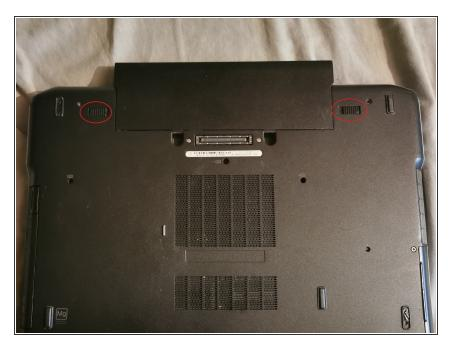
• Pull back the 2 battery tabs which are to the left and the right of the battery.
