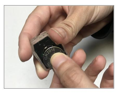
Insert the new battery into the bracket.
