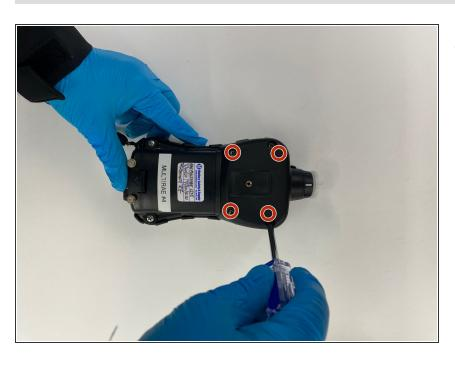
With the Phillips #0 screwdriver, remove all four 3 mm screws from the rear pump/sensor cover.
