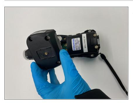
Remove the outer pump/sensor housing cover and set it aside.
