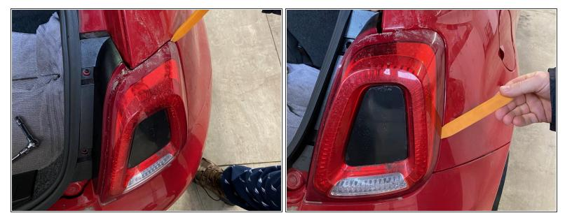
• Using a pry tool or something flat, carefully get in-between the light and the car and pry the light off.
