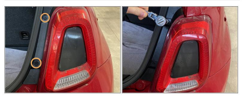
Remove the two 10 mm bolts to the side of the taillight.
