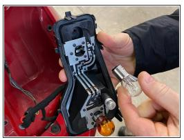
• Remove the burnt out bulb by pulling it out from the panel.
