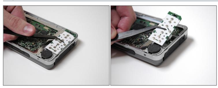
• Lift the keypad from the left side and use tweezers to slide it out to the left.
