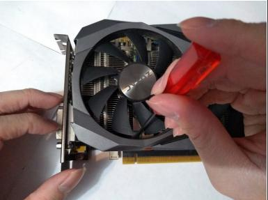
Use a Phillips #0 screwdriver to remove the two 4mm screws from the left side of the shroud.
