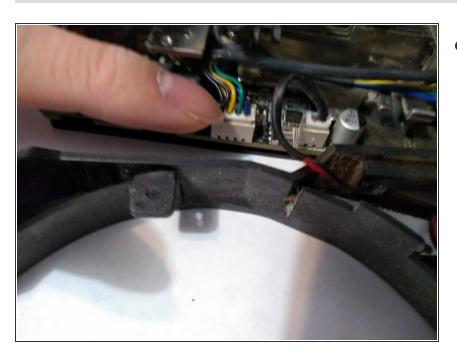
Reconnect the fan connector to its header.
