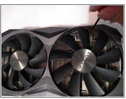
Place the shroud back over the heatsink and screw it back into place using a Phillips #0 screwdriver.
