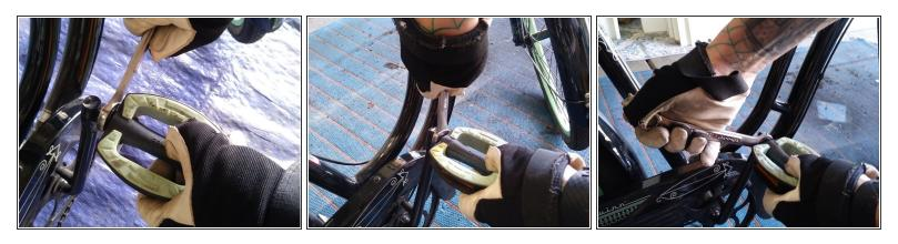
Holding the pedal with one hand, use a wrench on the base where it attaches to the crank and turn counter-clockwise.
