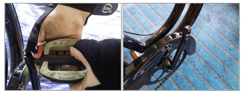
Using your hand, finish unscrewing the pedal.
