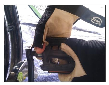
Using your fingers, begin screwing in the new pedal in a clockwise motion.
