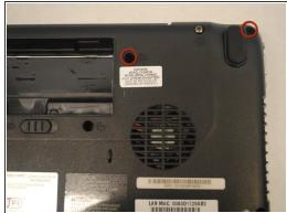
• Remove the four screws indicated in the photos using a Phillips 00 Screwdriver. Left to right: 6mm button-head, 3mm flat-head, 6mm button-head, 6mm button-head.
