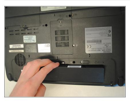
While holding the left lock, place your finger in the indentation next to the battery and lift the battery out.
