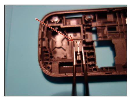
• Remove the vibracall engine with the tweezers
