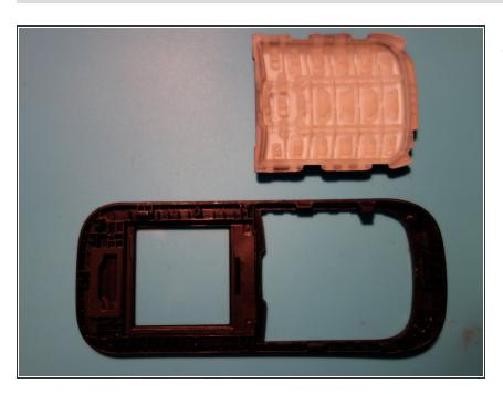
• Separate the rubber side of the keyboard from the rest of structure
