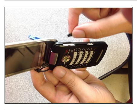
Once the keyboard is loosened, the button on the side of the phone may also release.
