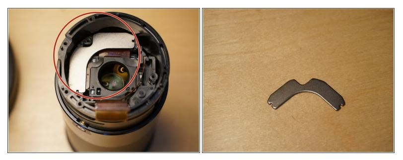
• Gently pry up magnetic OSS retaining bracket.
