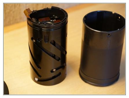
• Remove outer optical lens sleeve.
