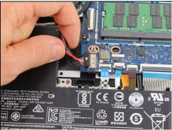
• Using your fingers, grasp the entire bundle of wires to pull the battery cable from its connector. This will cut off power to the motherboard.
