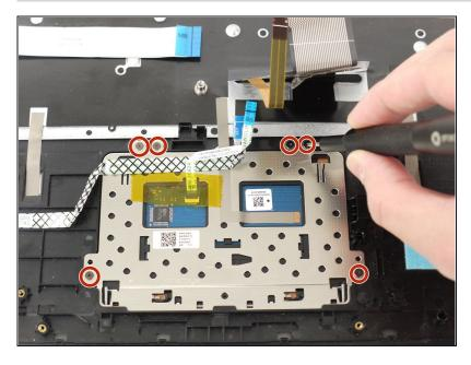
Using the JIS #000 screwdriver, remove six 2mm screws holding the trackpad down to the device.
