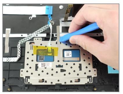
Using the plastic opening tool, remove the silver piece of tape holding the touchpad to the device.
