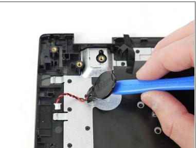
Using a plastic opening tool, pry the CMOS battery up and remove it from the device.
