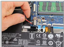
Using your fingers, grasp the entire bundle of wires to pull the battery cable from its connector.
