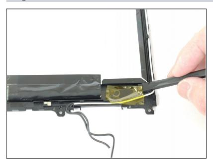
Using a spudger, remove the yellow tape on the bottom right corner of the screen.
