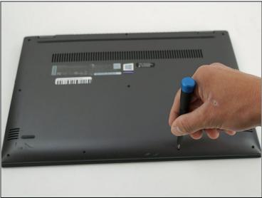
• Remove the ten 5 mm Phillips #00 screws that are holding the back panel on.
