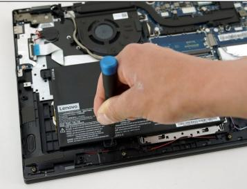
• Remove the two 5 mm Phillips #00 screws that secure the battery in place.
