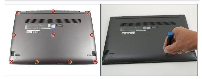
• Remove the ten 5 mm Phillips #00 screws that are holding the back panel on.
