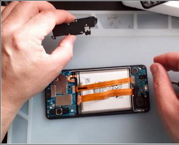
Use Phillips Screwdriver and plastic tool and remove the Sub board cover.
