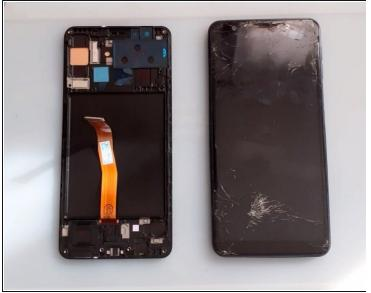
• It's better to use Display Assembly (Screen With Frame) to fix your broken device.
