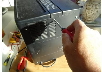
• The rear panel and side panels are attached with six phillips screws #2. Screw them out.
