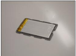
Remove the battery from the casing by bending the sides. The battery should pop out.
