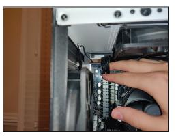
• Unplug the various power cables. These include the Mainbords big 24 pin cable, the processor's power cable, the graphics card power cable, the SATA cables for the fan control, and the motherboard's power cable
