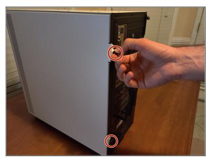
Remove the side panel by unscrewing the captive thumb screws keeping it in place.
