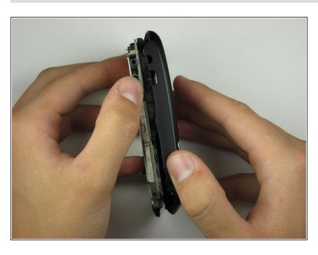
To remove the phone's internals, start by loosening one side by pulling gently.
