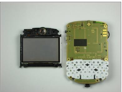
With the clip unhooked, gently separate the display from the phone internals by pulling.
