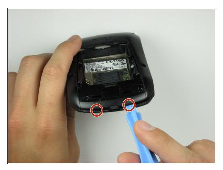
Use the plastic opening tool to apply pressure on the two clips that are located at the bottom of the phone.
