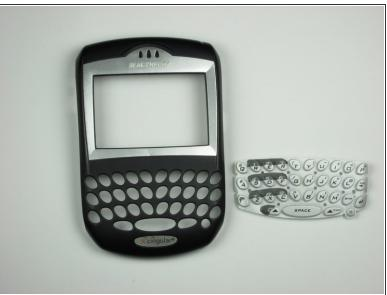
Peel off the rubber keypad buttons from the face plate.
