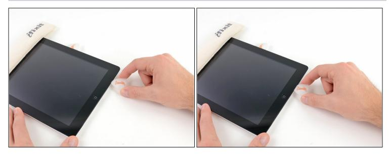
This step requires you to move the opening pick along the bottom right edge of the front panel. The Wi-Fi antenna is very close to the corner and is easily severed if the adhesive is released improperly.
