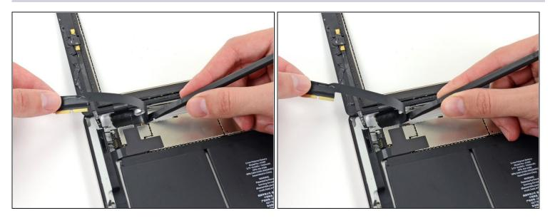
• Peel back the digitizer ribbon cable and use the flat end of a spudger to release the adhesive securing the cable to the rear aluminum case.
