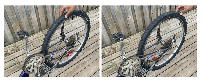
Rotate the wheel again to ensure the brake did not change positions while you were tightening it.
