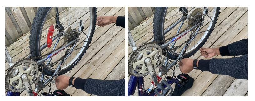
Rotate the bicycle tire to ensure the brake is no longer rubbing against the rim.
