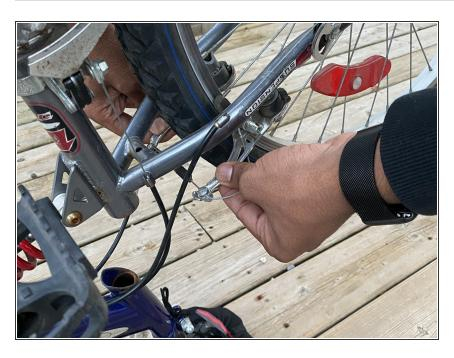
Shift the brake so that the pad no longer makes contact with the rim.
