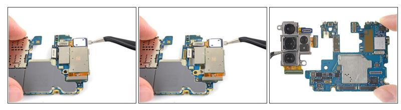
• Use a pair of tweezers or your fingers to remove the rear camera module.
