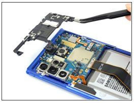
Use a pair of tweezers to pivot the top plastic cover up and off of the phone.
