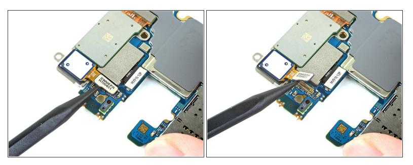
Use the pointed end of a spudger to disconnect the top camera connector.
