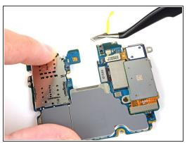
• Use a pair of tweezers to remove the small piece of tape covering the middle camera connector.
