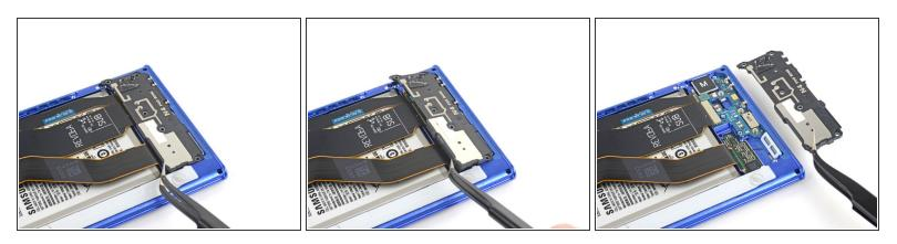
Use a pair of tweezers to remove the loudspeaker.
